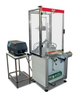
Semi-automatic machine to apply one elastic pen loop onto agenda and diary cases or onto already cased-in products by hot-melt.
