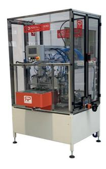
Semi-automatic machine to thread and glue one flat elastic band onto laying flat agenda and diary cases.
