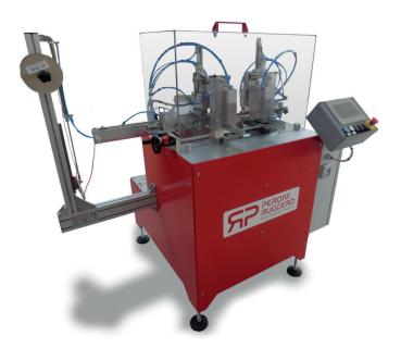
Semi-automatic machine in simplified version to thread and glue one flat elastic band onto laying flat agenda and diary cases.
