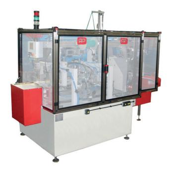
Semi-automatic machine to apply one flat elastic band onto spiral notebooks by 2 rivets or evelets.
