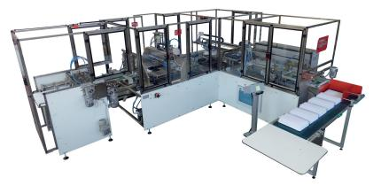
Automatic line to assemble folders in one single die-cut piece, having one straight round elastic band with 2 rounded metal tags.
