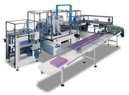
Automatic line for assembling folders with round straight elastic band having 2 round metal tags, equipped with units for side flap application and for collecting/delivery of the final products in piles.
