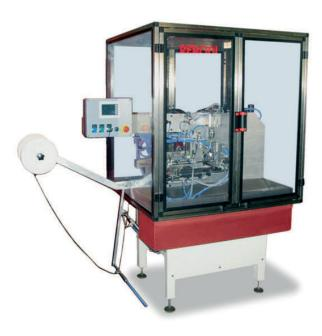
Automatic equipment for the production of round elastics closed in ring-shape.
