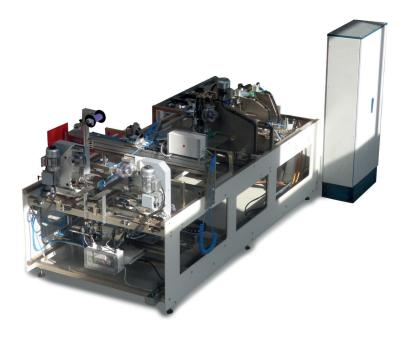
Automatic machine for assembling folders with flat criss-cross elastic band fastened by metal eyelets.
