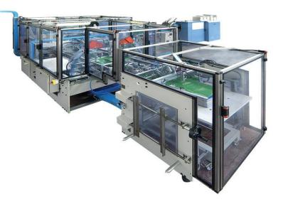
Automatic line for assembling folders with straight and criss-cross elastic band having two rounded metal tags.
