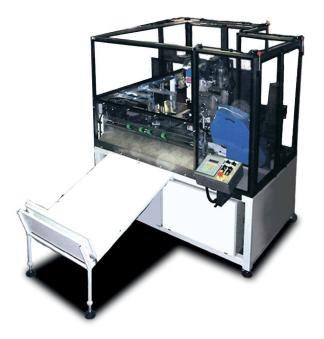
Half-automatic machine for the application of snap fasteners by means of one revolving assembly platform.
