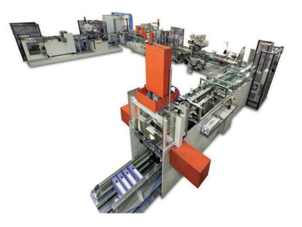
Automatic line for assembling document holding boxes in polypropylene, equipped with hot creaser, pocket welding and paper label positioning units on box spine and front, application of 1 finger eyelet, fastening of one piece of selfadhesive velcro and one metal clip, box folding and shaping devices by ultrasounds.
