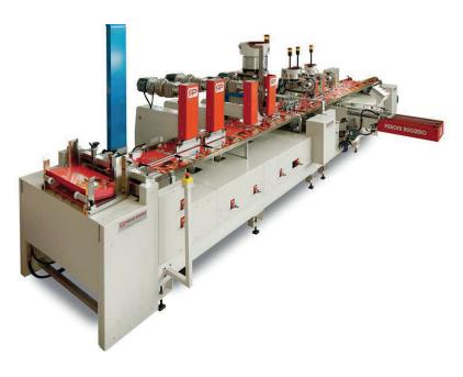
Fully automatic line to crease (2 creases), to set 1 finger ring and to rivet ring metals (3rd rivet included)
