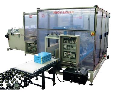
Automatic line for creasing, riveting two side flaps and fastening one elastic band 15 mm wide, supplied with folding and elastic rotating unit for map closing.
