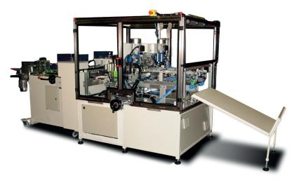
Automatic line for creasing and riveting two side flaps on folders.
