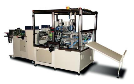
Automatic line for creasing folders, automatically riveting two side flaps and fastening one elastic band 15 mm wide. **(CORD-R+FLAP15+ELAP15)**
