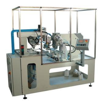
Half-automatic machine to apply one string onto wall calendars by using Nr. 02 eyelets.
