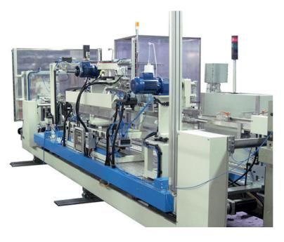
Fully automatic line to apply one string onto wall calendars by using Nr. 02 metal eyelets.
