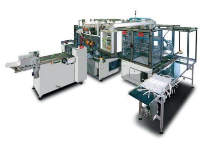
Automatic line for assembling files having 6 tapes (fastened by metal eyelets), supplied with board case creasing unit.
