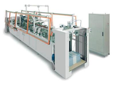
Automatic line for assembling files having 6 glued tapes. **HOT-MELT** gluing system
