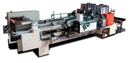
Automatic line for manufacturing suspension files with metal or plastic bars. Bars feeding by hand. Bar applying in automatic
