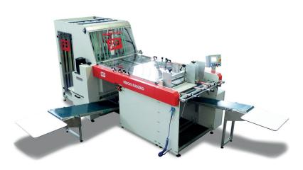
Automatic rotative grooving machine for board cases, supplied with a double feeder, grooving unit for "V" and "U" cuts, in-line corner cutting device.
