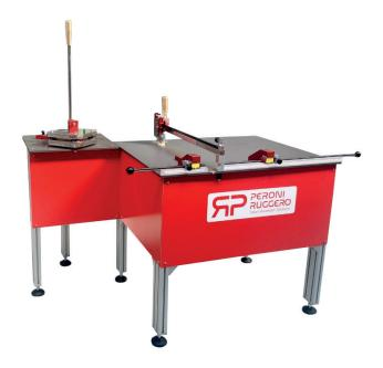
Manual equipment to cut the corners of the box blanks and make V & U-shape grooves. Ideal for mock-up samples and short runs.
