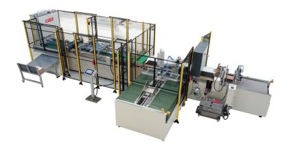
Automatic casemaking & lining machine to manufacture covers both in one piece and in several panels.
