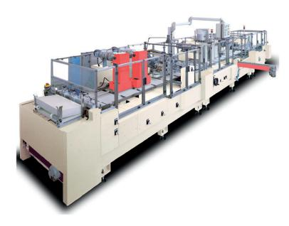
Fully automatic modular line for lever-arch file assembling (high speed equipment).
