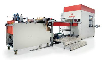
Gluing unit with automatic viscometer; Manual positioning of the box onto the glued paper with mechanical centering device. Automatic centering & traslation of the materials to the automatic wrapping unit by telescopic conveyor tape;
