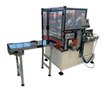
Automatic machine to weld plastic pockets onto file spines, supplied with paper label positioning unit.
