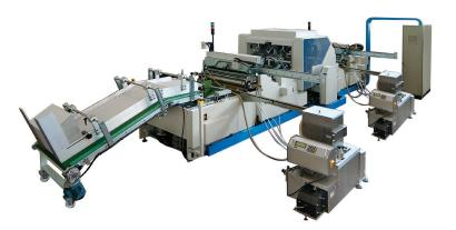
Automatic case-making & lining machine in line (hot animal glue & cold vinylic glue).
