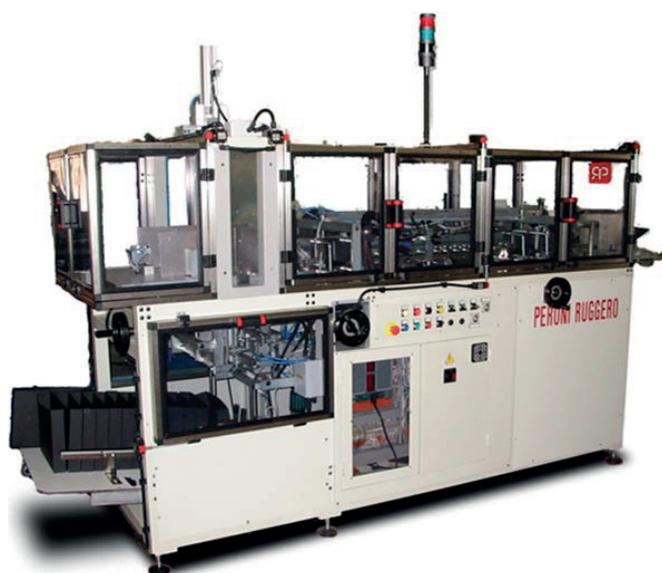
Automatic lines to form and to glue file and book slipcases with Nr. 02 folded-in flaps – HOT-MELT gluing system.
