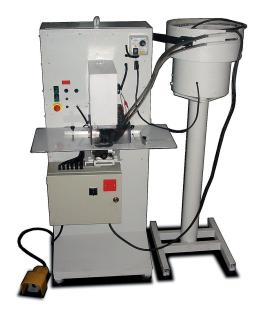
Motor driven manual machine to apply nr. 01 Finger Ring - Board feeding by hand -Punching and applying operation without board shifting. Eyelet feeding via vibrator.
