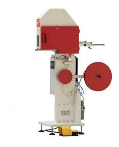
Manual unit for the automatic application of one self-adhesive thermal tape as used to keep rigid box corners closed.
