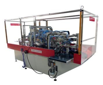
Automatic machine to thread and glue one flat elastic band onto laying flat agenda and diary cases.
