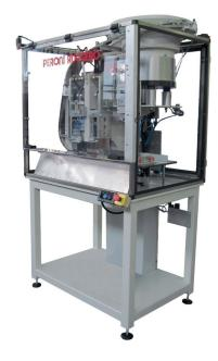
Motor driven manual machine to apply nr. 02 Rado eyelets – Board feeding by hand – Punching and applying operation without board shifting.
