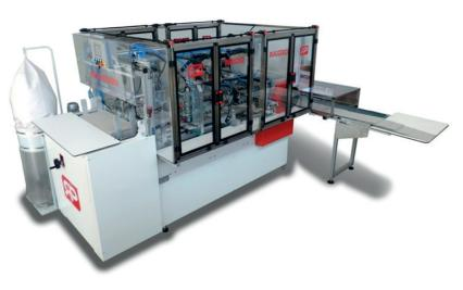
Fully automatic machine to groove board seats and to apply 2 or 4 magnets by using hot-melt glue.
