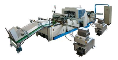
Automatic case-making & lining machine in line (hot animal glue & cold vinylic glue).
