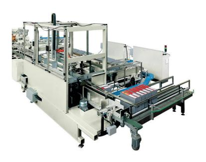
Automatic insertion unit of lever-arch files into their slipcases
