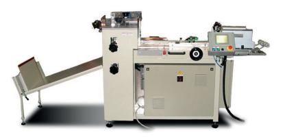
Automatic machine for multiple creases, supplied with automatic board feeding unit.
