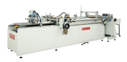
Semi-automatic gluing machine able to glue paper, laminated paper, cardboard, paper-based fabric and thanks to its versatility, it's possible to produce a wide range of products such as one-piece ring binders and multi-pieces covers, board games and photo albums, displays and calendars, rigid and collapsible boxes, folders and more.
